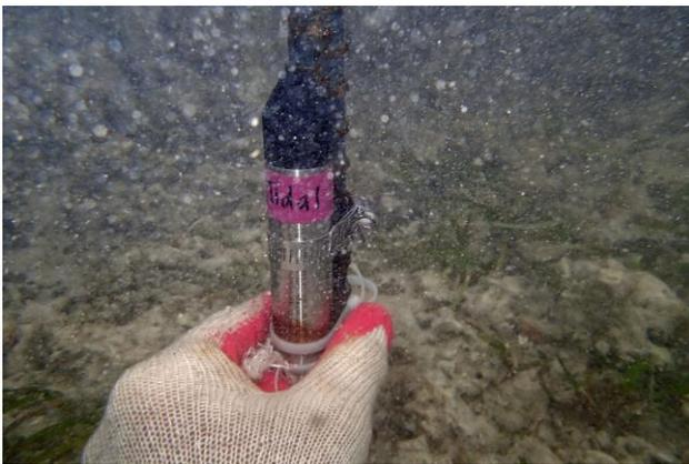
**Figure 2:** The water level logger tied to the rebar with an adjustable metal screw bolt clamp tie and a zip tie.
