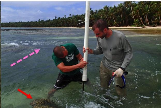
**Figure 3:** Placing the PVC tube over the rebar. The gauge was set up behind a coral pinnacle (red arrow) in the wave shadow. The pink arrow shows the wave direction. *Photo credit: Maria Kottermair*
